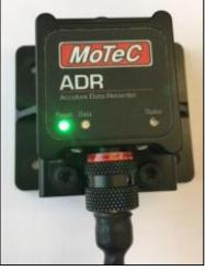
The ADR is mounted to a bespoke bracket by three screws. In-turn, the bracket is mounted via riveted nuts and oval-head screws towards the rear of the body-shell's centre tunnel forward of the shifting valve-block, as depicted in the images to the left. The position of the ADR installation in the car shall under no circumstance be altered.
